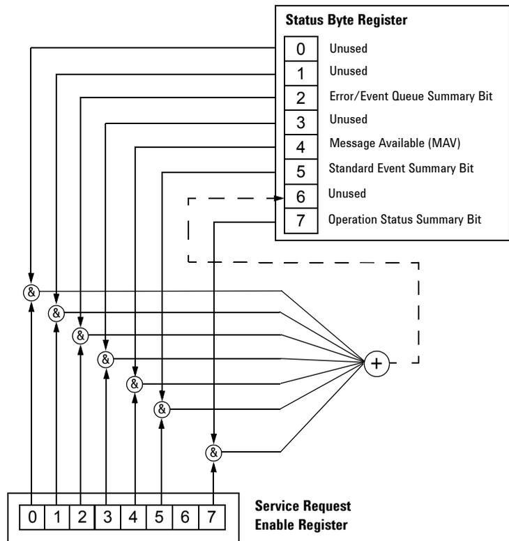
The RQS bit is read and reset by a serial poll. The same bit position (MSS) is read, non-destructively by the **\*STB?** command. If you serial poll bit 6 it is read as RQS, but if you send **\*STB** it reads bit 6 as MSS. For more information refer to IEEE 488.2 standards, section 11.
