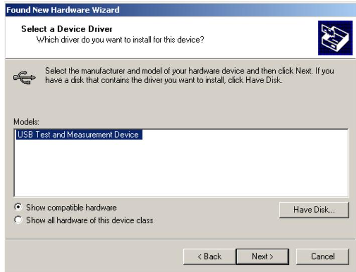
The wizard will guide you through the rest of installation till the driver is installed. Run Keysight IO libraries suite, the analyzer will be detected automatically.
